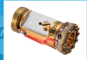
Liquid Nitrogen Cooled JFET Module for Energy Dispersive X-Ray (EDX) Applications.
